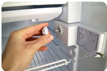
3) Remove the thermostat knob
