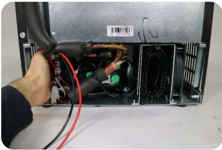
2) Pull out the cooling unit
