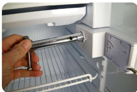
4) Unscrew the screw-nut fixing the thermostat
