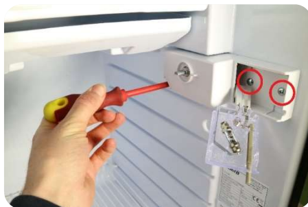
5) Push the button and pull out the plastic glass to remove it, then unscrew the ceiling light
