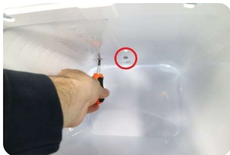
2) Unscrew the bracket fixing the thermostat sensor (2 screws on the evaporator)
