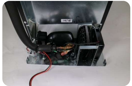
2) Pull out the cooling unit
