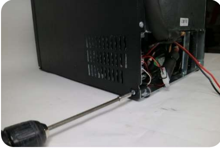
1) Unscrew the cooling unit (2 screws each side)
