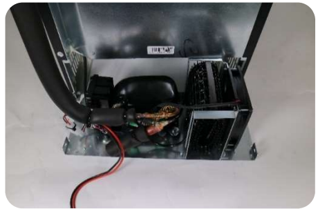
2) Pull out the cooling unit
