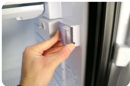
5) Push the button and pull out the plastic glass to remove it, then unscrew the ceiling light
