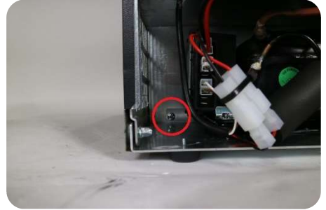
1) Unscrew the cooling unit (2 screws each side)
