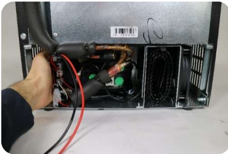
2) Pull out the cooling unit
