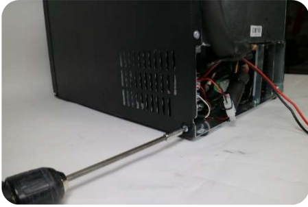
1) Unscrew the cooling unit (2 screws each side)
