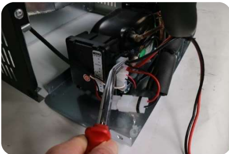
3) Disconnect all the wires from the ECU unscrew the screw fixing the ECU
