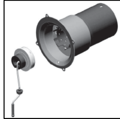
Figure 6: Evaporator Mount with Combustion Pipe (Benzin)
