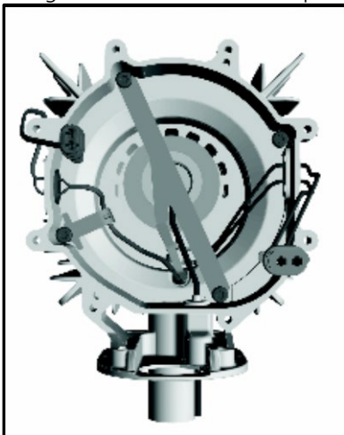
Figure 36: Top view of heat exchanger
