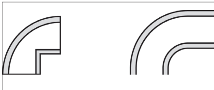
Fig. 41 Elbows: cast pipe (left) and bent pipe (right)
